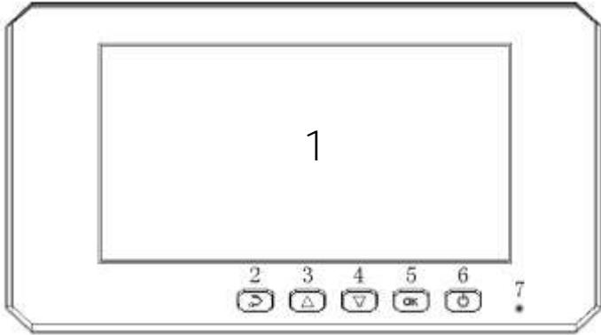
1. 7 inch LCD: displays information such as the number of passengers, alarms, detection signal strength, time, and working channel.
