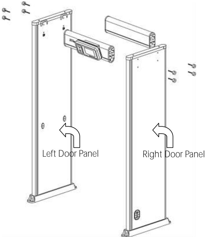
1. Remove the package of the host, beams, and door panels.
